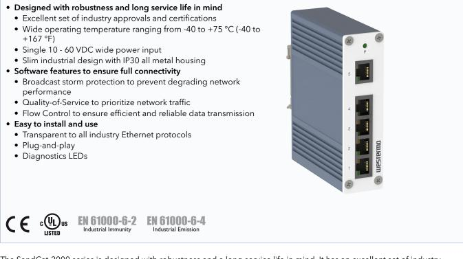
The SandCat-2000 series is designed with robustness and a long service life in mind. It has an excellent set of industry approvals and certifications, ensuring its reliability and performance. The devices operate in a wide temperature range from -40 to +75 °C (-40 to +167 °F), making them suitable for harsh industrial environments.
