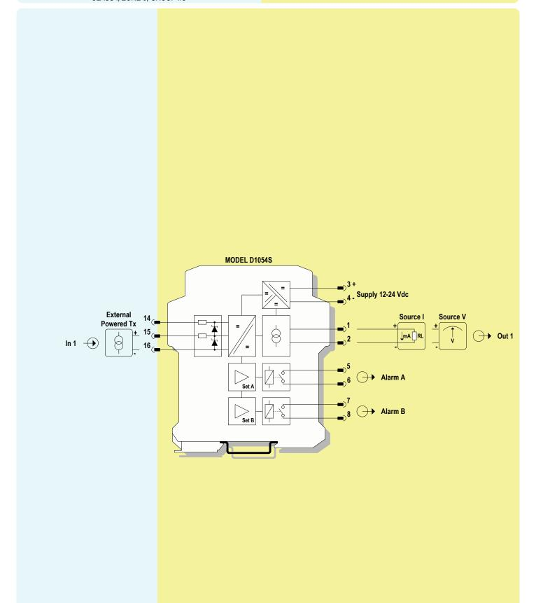
For SIL applications, alarm contacts must be used in series with equal configuration. Relay contacts shown in de-energized position.
