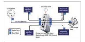
a high level of synchronization within an industrial motion-control environment with a minimum use of network and computing resources. The protocol helps for sequencing event measurements, scheduling outputs, synchronizing actuation, time-stamping, coordinating event records, etc.
