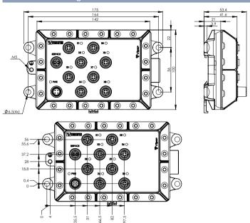
Weight 0.9 kg Degree of protection IP65
